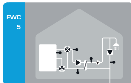
Fresh water system with mixing valve on the primary side, zone valve and circulation pump
