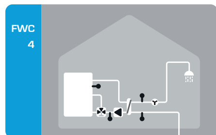
Fresh water system with zone valve
