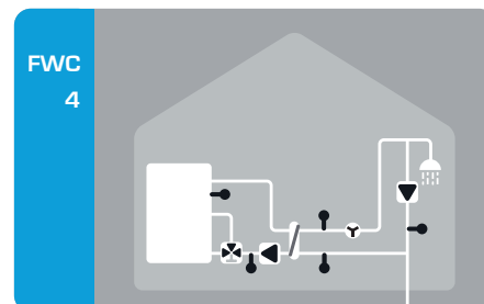
Fresh water system with zone valve and circulation pump
