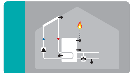
Solar with thermostat and return flow increase
